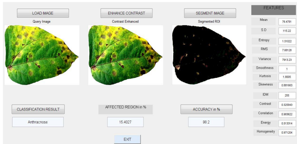
Figure 3: System shows leaf disease detection of P. vulgaris using digital image processing techniques
